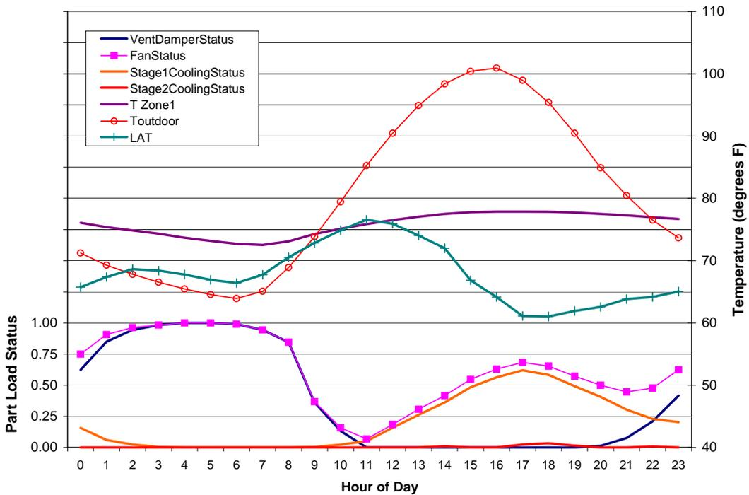
Figure 12 plots similar data to that shown in Figure 11 for the NB2 control with variable speed capability. Data included are from September 17<sup>th</sup> through October 10<sup>th</sup> and represents considerably cooler weather conditions. NightBreeze operation largely occurred from 8 PM to midnight during this milder weather<sup>8</sup>.
