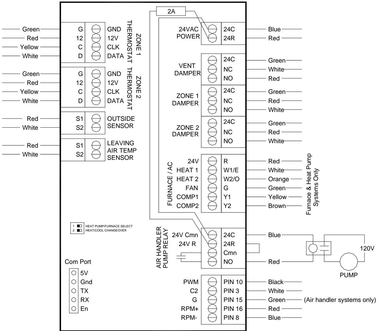
ALTERNATE PUMP CONTROL WIRING FOR SWITCHING RELAY
